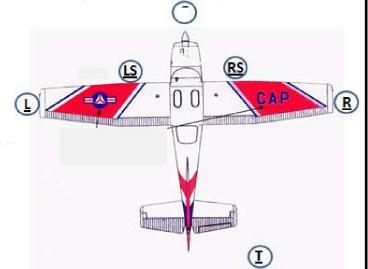
The Movement Team Leader (MTL) is always positioned at the nose of the aircraft. Other members should be placed relevant to the highest risk to the aircraft being moved.
